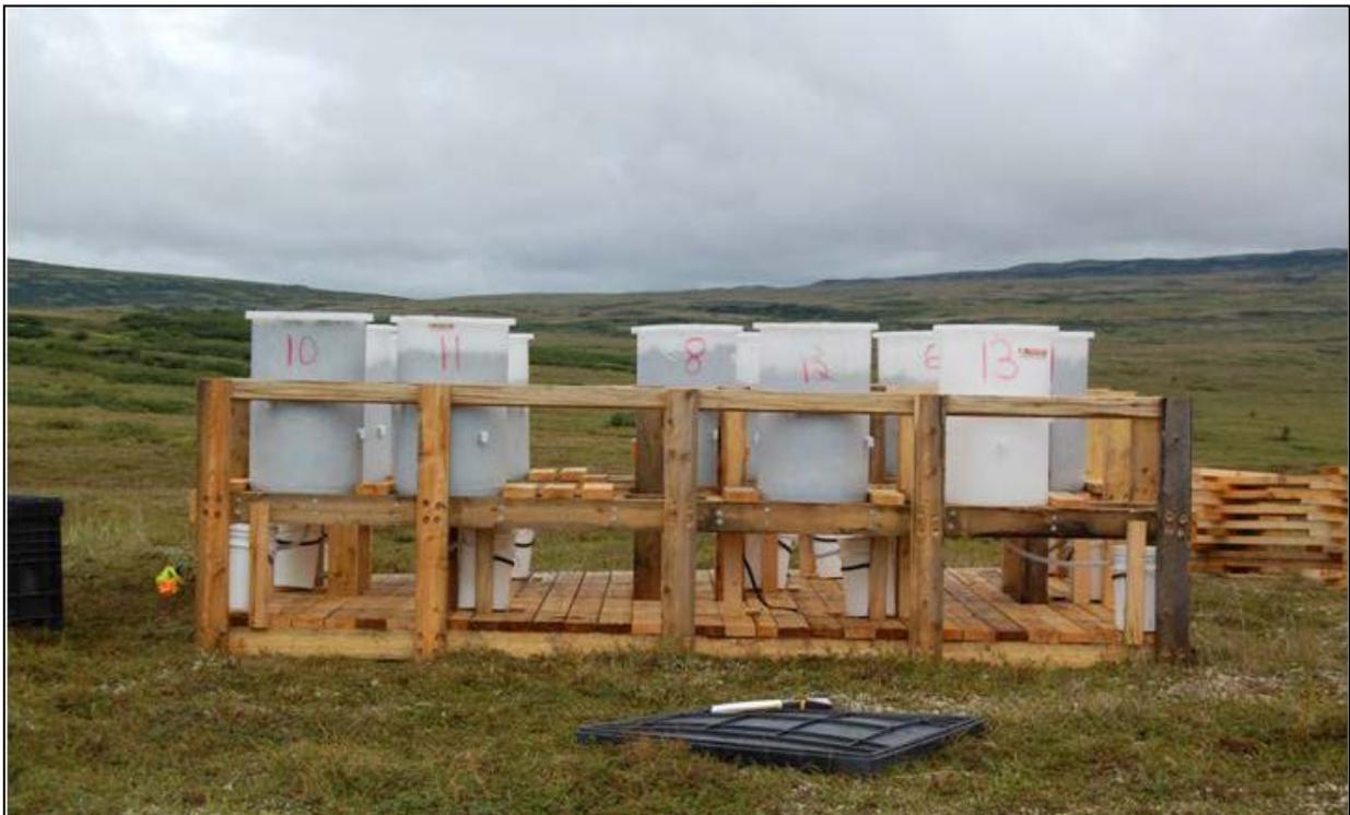
**PHOTO 11-2.** Field weathering (barrel) tests were constructed on-site.
