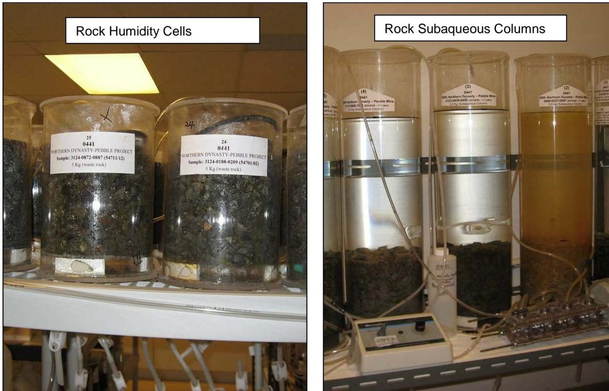
**PHOTO 11-1.** Laboratory tests included humidity cells and subaqueous columns.
