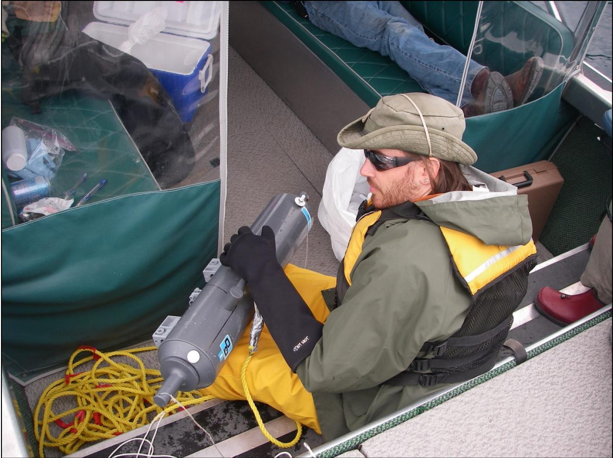
Water sampling using the Niskin sampler.
