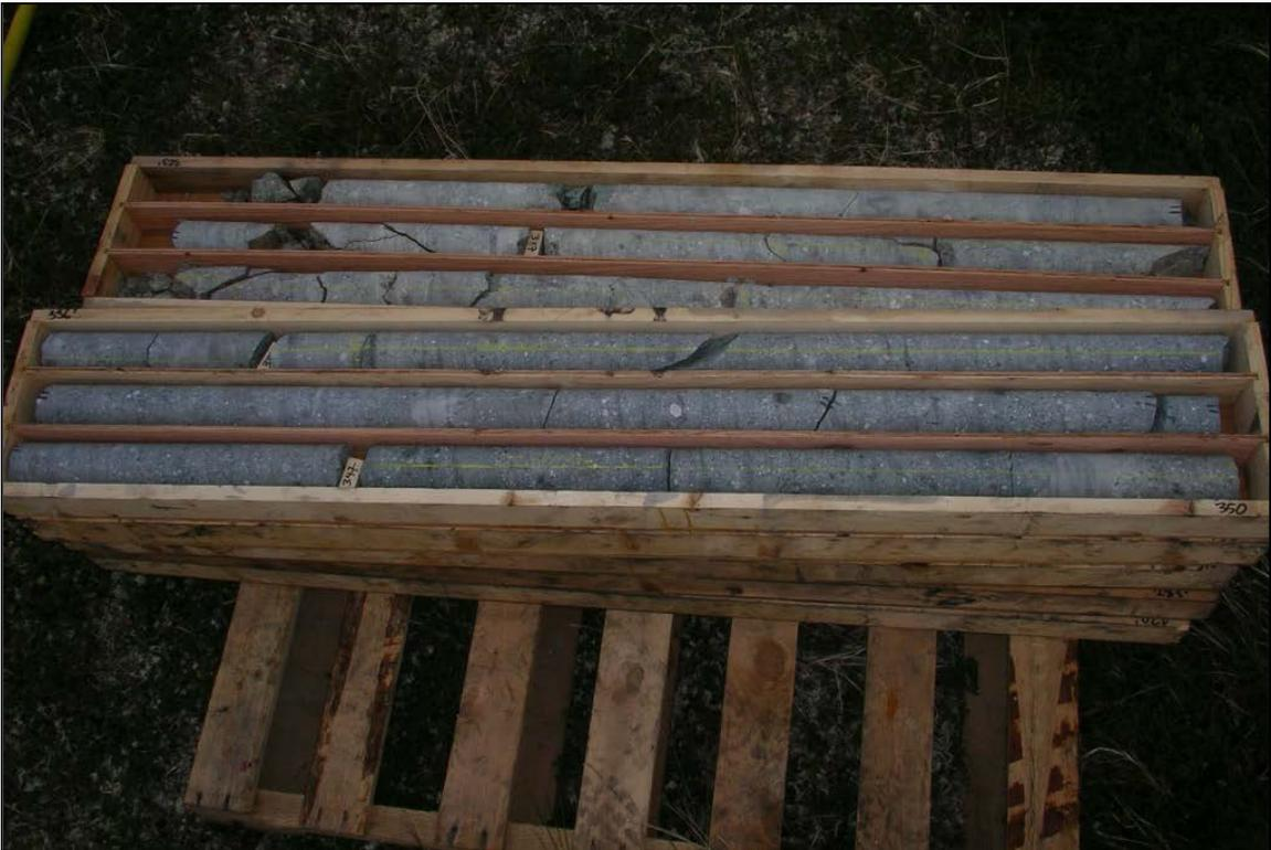
Typical bedrock cores from exploration/geotechnical drilling.
