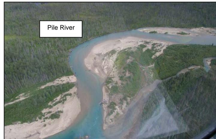
**PHOTO 4-4.** Transportation-corridor study area, typical braided channel pattern in the Pile River near the mouth, July 2008.
