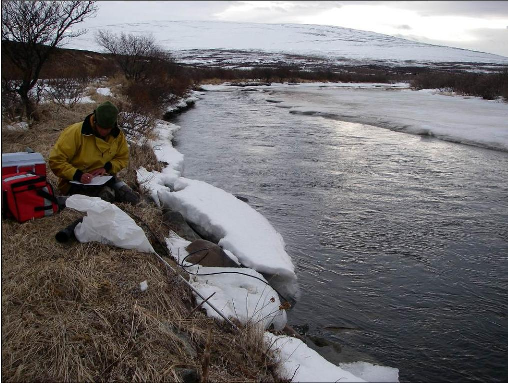
Using a multi-probe meter to measure in situ water conditions in the North Fork Kaktuli River during early spring.
