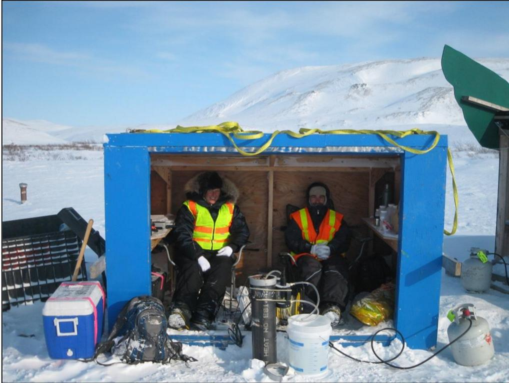
Collecting groundwater samples and measuring in situ water conditions in March.
